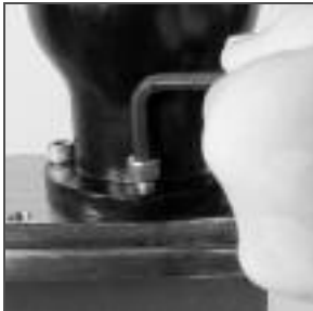
Remove only two actuator bolts
