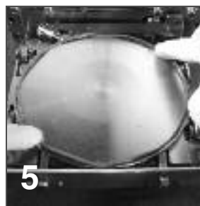
5 Press straight down without twisting the O-ring.
