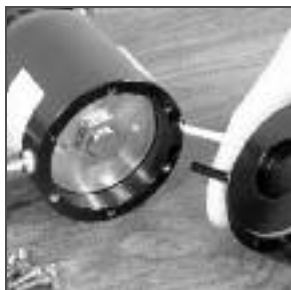
Position Indicator partially out
