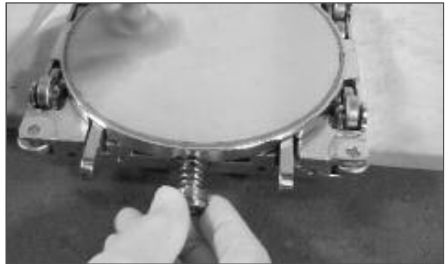
Install the gate spring
