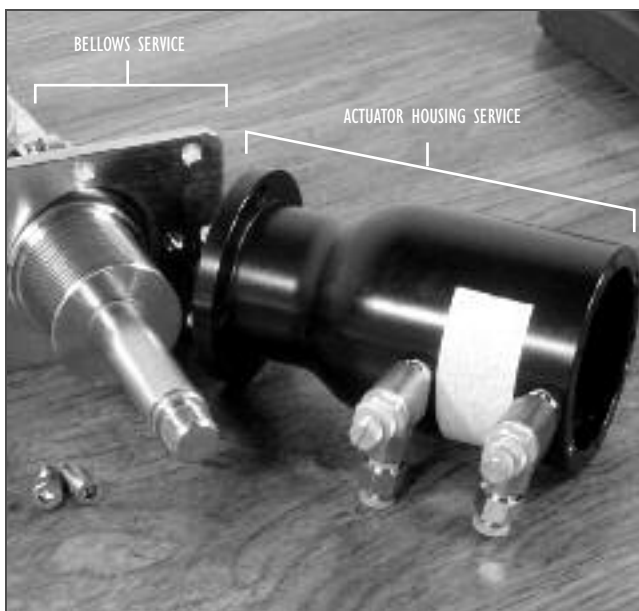
REMOVE & SEPARATE Actuator Housing
