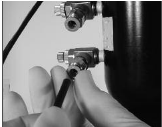
Air line installation
