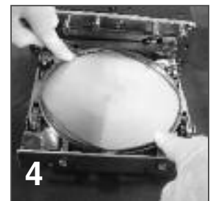
4 Continue pressing O-ring into groove at 180°-apart intervals.
